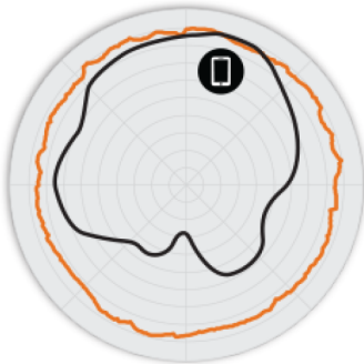
Figure 2. T750 2.4GHz Azimuth Antenna Patterns
