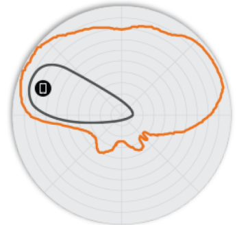
Figure 5. T750 5GHz Elevation Antenna Patterns
