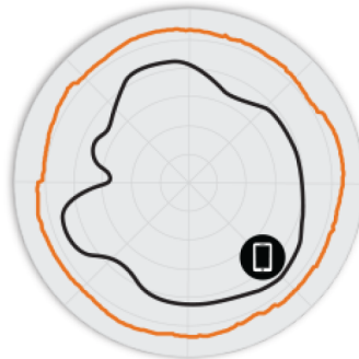
Figure 3. T750 5GHz Azimuth Antenna Patterns
